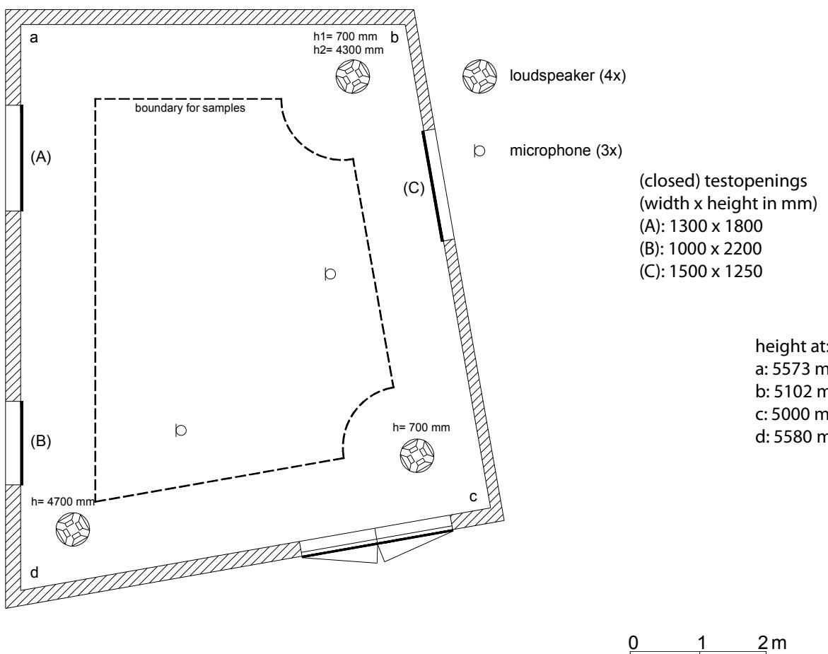
**MEASUREMENT OF SOUND ABSORPTION IN A REVERBERATION ROOM
