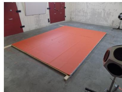
Absorb, versie 5.8.4 mode 7, PM: JK, file: a3233 E#1-36 F#186-221 A#2222 T<sub>1</sub> = 17,1 °C T<sub>2</sub> = 17,2 °C P<sub>1</sub> = 102,8 kPa P<sub>2</sub> = 102,7 kPa h<sub>1</sub> = 53,1 % h<sub>2</sub> = 53,0 %volume reverberation room: 214 m<sup>3</sup>surface area sample: 11,7 m<sup>2</sup>
