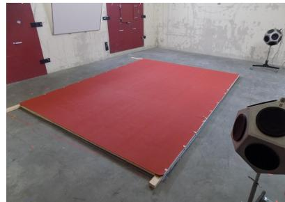
Absorb, versie 5.8.4 mode 7, RM: JK, file: a3233 E#:1-36 F#:149-184 A#:185 T<sub>1</sub> = 17,1 °C T<sub>2</sub> = 17,3 °C P<sub>1</sub> = 1028 kPa P<sub>2</sub> = 1028 kPa h<sub>1</sub> = 53,1 % h<sub>2</sub> = 52,3 %volume reverberation room: 214 m<sup>3</sup>surface area sample: 11,7 m<sup>2</sup>
